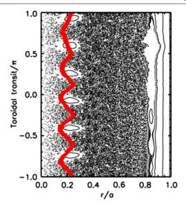
**Figure 5.** A puncture plot of magnetic field lines (dots) and a fast-ion orbit guiding centre (solid line) from a simulation of a standard RFP discharge. Full orbit simulation shows that fast-ion drift orbits do not follow the magnetic field lines, resulting in different rotational transforms for fast ions and magnetic field lines.
