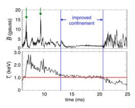
**Figure 2.** (Top) Magnetic fluctuation amplitude is reduced during the improved-confinement period. (Bottom)  $C^{+6}$  impurity ion temperature is sustained at approximately 1 keV. The two vertical arrows mark reconnection events during which ions are strongly heated.
