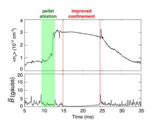
**Figure 6.** Injection of a frozen deuterium pellet at the start of an improved-confinement period triples the line-average electron density while magnetic fluctuations are maintained at a reduced level. Pellet ablation occurs during the shaded time, and the improved-confinement period is delimited by vertical lines.
