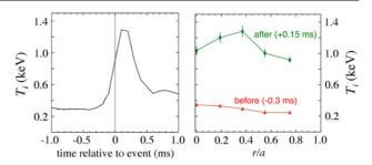
**Figure 1.** Left: the impurity ( $C^{+6}$ ) ion temperature at r/a = 0.37 through a global reconnection event. Right: radial profiles of the impurity ion temperature before and after a global reconnection event.
