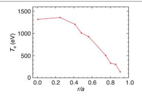
Figure 3. Electron temperature as measured by Thomson scattering is also greater than 1 keV during improved-confinement discharges.
