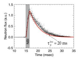
**Figure 4.** Comparison of measured neutron signal (dots) and modelling (solid line). The shaded area represents the neutral beam injection duration. The solid  $\tau_{\rm fi}^{\rm loss} = 20$  ms line is a result of modelling with classical fast-ion slowing down and 20 ms fast-ion confinement time.
